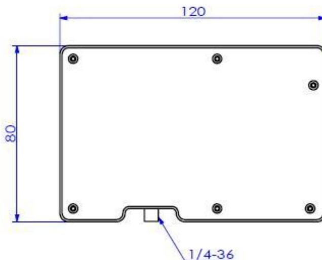
**The size of ATP5001 micro spectrometer**
